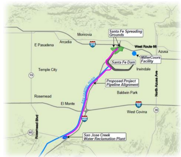
Figure 6-1. IRRP Proposed Pipeline Alignment.
